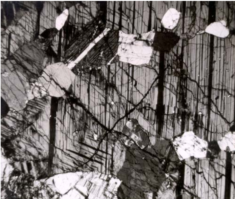
Figure 2: Photomicrograph of thin section of 15415, crossed polarizers, showing polysynthetic twinning in mildly shocked plagioclase and trigonal grain boundaries. Field of view is 3 mm. NASA # S71-52630
