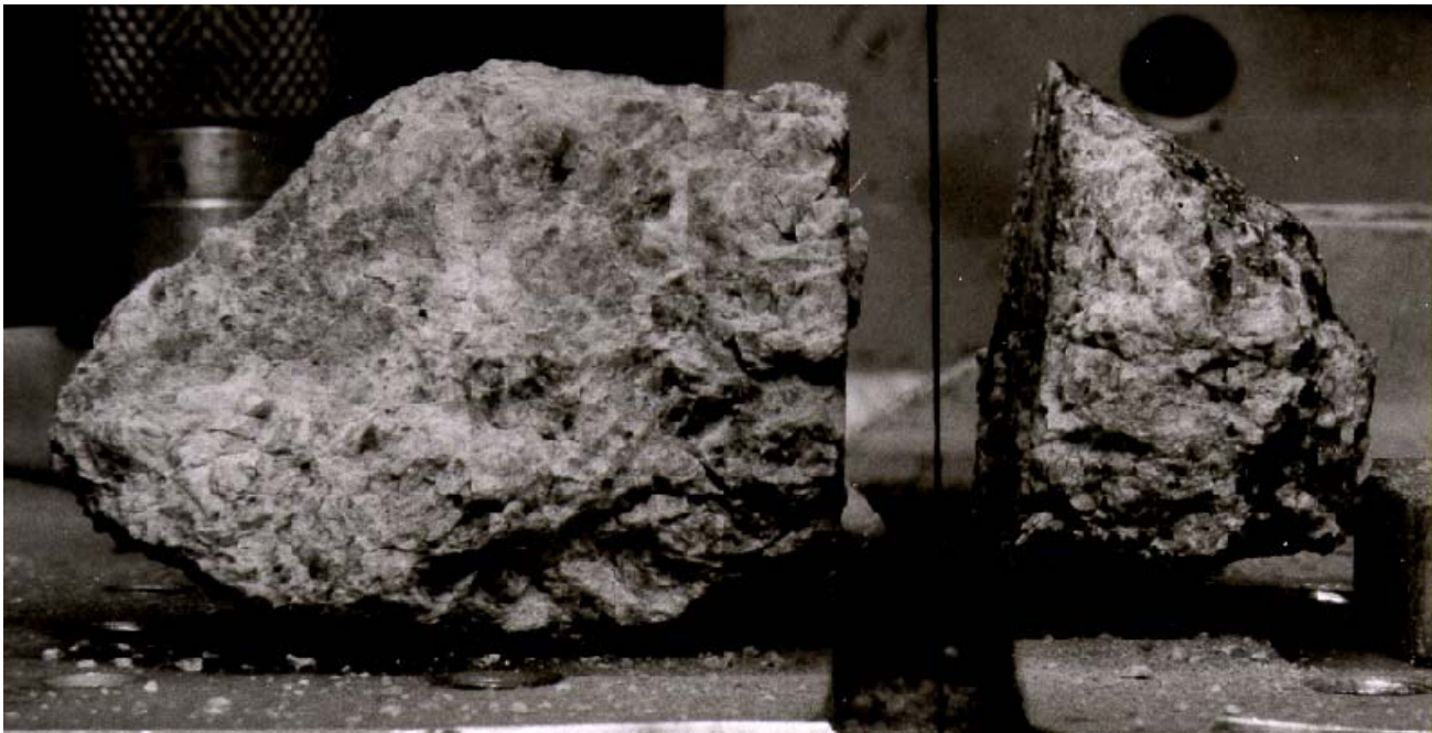
Figure 8: First saw cut of 15415,0 yielding 15415,33. NASA photo # S712-15899. Sample is about 3 inches high.
