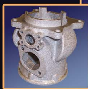
Titanium can be used to make lightweight yet very strong mechanical parts like this spacecraft component.
